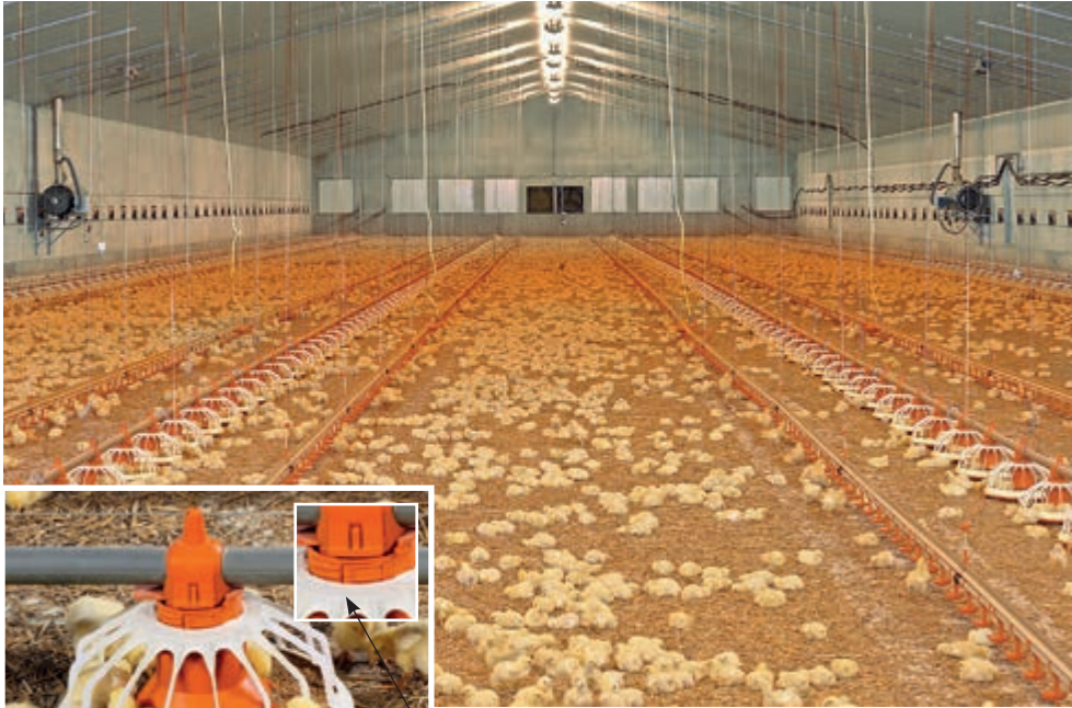
FLUXX 360 with corrugated bottom, feed shut-off and 16-arm grill The arrow indicates the selected feed level (there are 7 or 8 levels) -> easy to read
